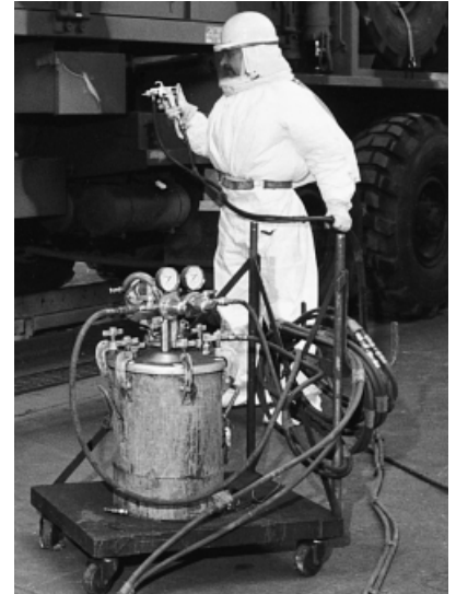
A typical industrial paint "kitchen" utilizes several sizes and types of tanks.
