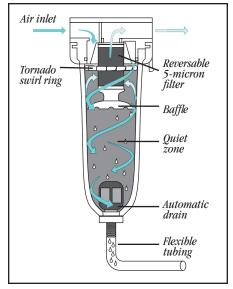
Tornado-like swirling action removes moisture which collects in the baffled "quiet zone." The reusable 5-micron filter catches smaller impurities. Accumulated liquid is carried away by the automatic drain.
